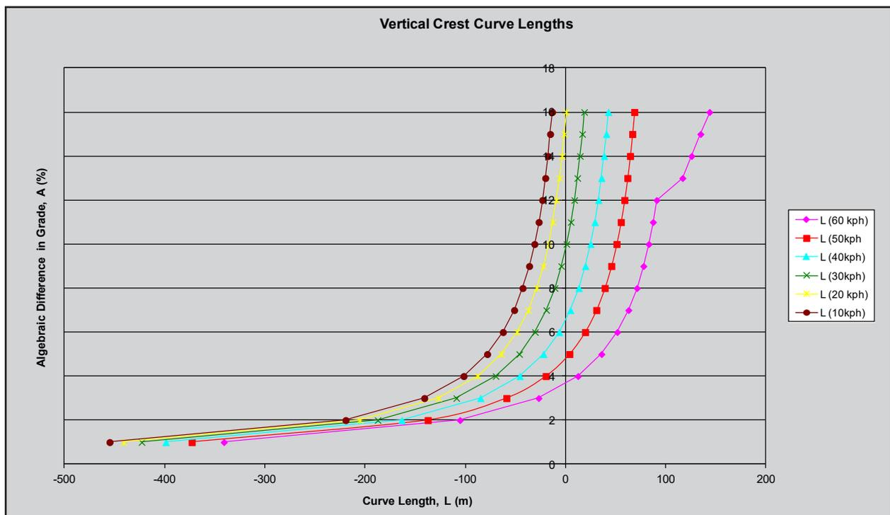
Figure 5: Vertical Crest Curve Lengths
