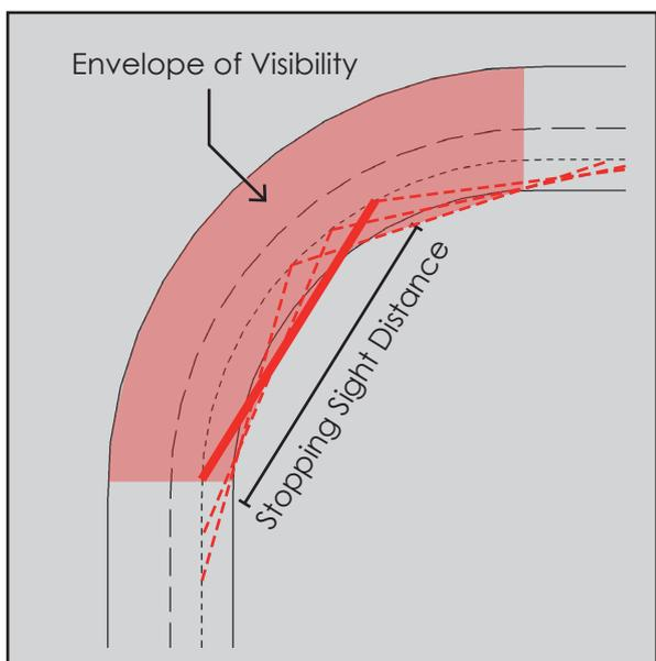
Figure 2: Forward Visibility at Horizontal Curves
