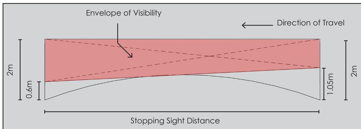
Figure 3: Visibility Envelope in the Vertical Plane
