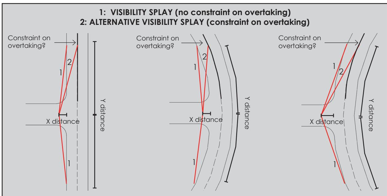
Figure 4: Visibility Splays at Junctions
